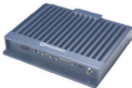
The Qualcomm QDEC-1000 digital cinema decoder is about the same size as an A4 sheet of paper. It may not look particularly impressive, but there must be a lot going on in there because it draws up to 10A at 5V! Picture resolution is adjustable up to 2560x1080 pixels.
