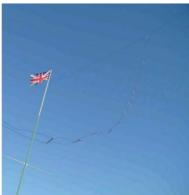
G3LDO's own '50-50' antenna - a 50ft length of wire centre fed with home-made twin-line feeder. The green and white pole flying the union flag is part of a different antenna system.
