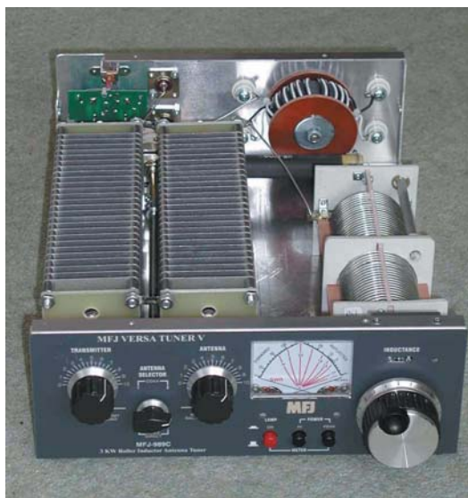
MFJ Versa Tuner V (989C), which rated well on GW3NDR's efficiency test. Note that the components are quite chunky to handle high power, which may have contributed to good performance.
